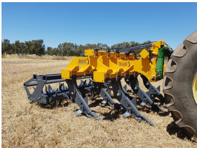
Example delving deep rippers: Left : with low rake angle flat face tines set at narrow spacing (Image: FarmTech Machinery) ; Right : with additional mixing top-plates fitted (Image: University of South Australia)
