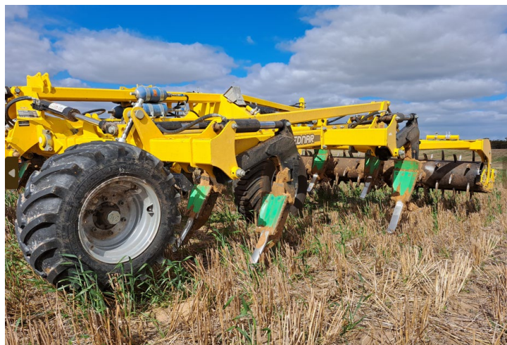
Example delving deep rippers: Left : with low rake angle flat face tines set at narrow spacing (Image: FarmTech Machinery) ; Right : with additional mixing top-plates fitted (Image: University of South Australia)
