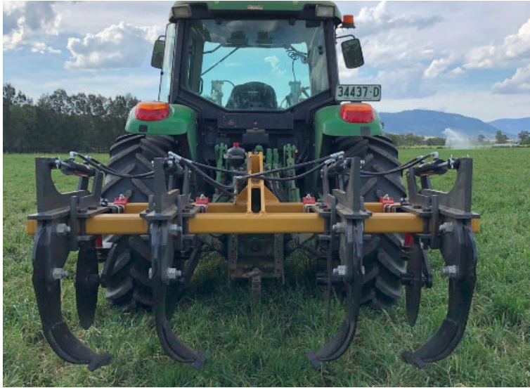
Curved slanted tines minimise surface disturbance and benefit from slightly lower draft. Image: Williamson-Agri
