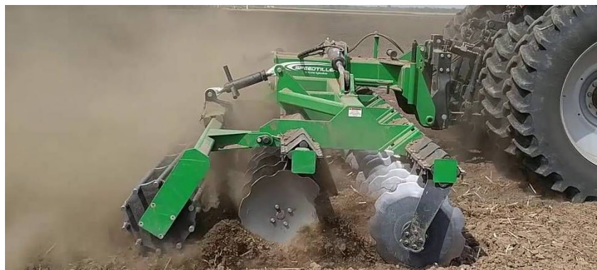
Top: Offset disc harrows, trailed with in-frame carrier axle (Image: Gessner Pty Ltd) ; Bottom: compact disc harrows in operation (Image: K-Line Agriculture)
