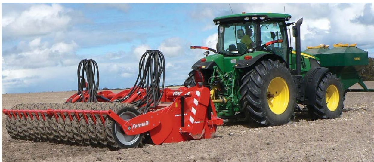
Rotary spaders use sets of winged blades (inset) to loosen and mix the soil profile down to 35-40cm depth (Image: Grocock Soil Improvement)
