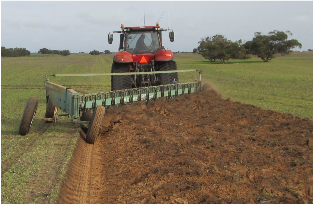
Plozza disc modified 5GP trailed one-way plough operating at 32cm depth (Image: University of South Australia)
